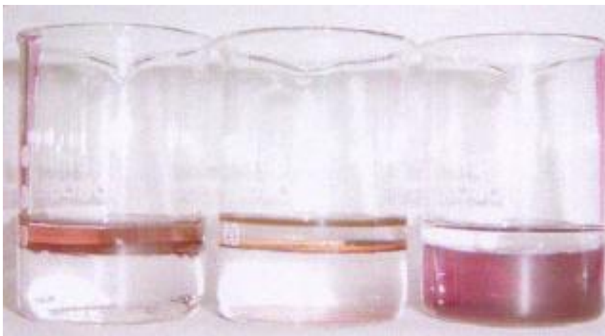
Figure 35. (Middle) Nanocrystals of Au formed at the toluene–water interface. (Left) When dodecanethiol is added to the toluene layer, the Au nanocrystals form an organosol. (Right) When mercaptoundecanoic acid is added to the water layer, the Au nanocrystals produce a hydrosol.
