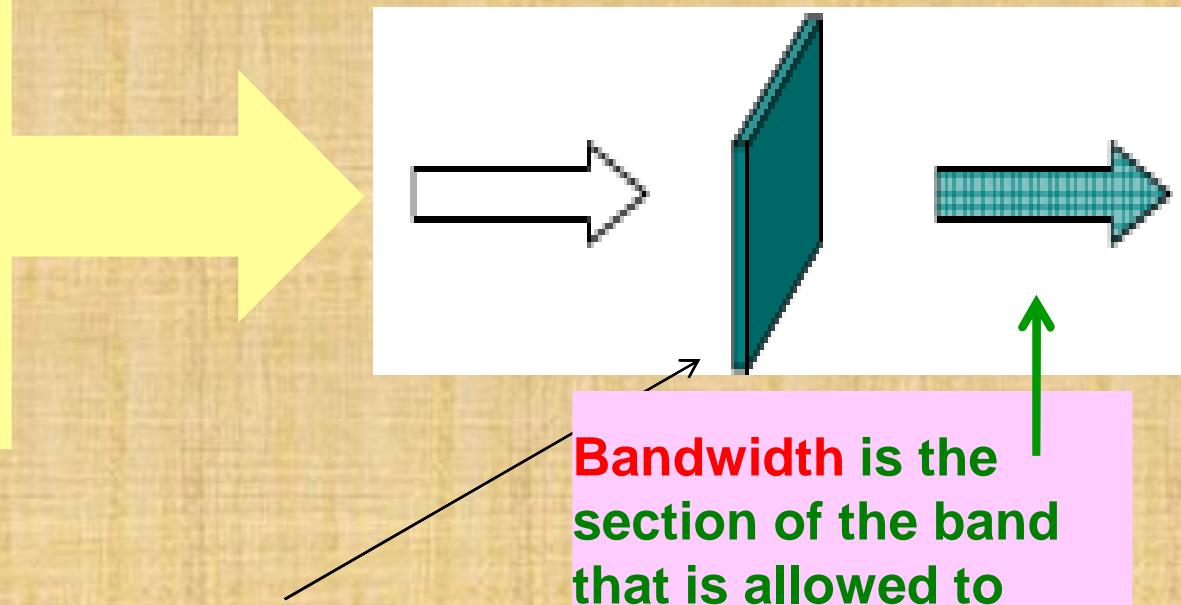
**Bandwidth** is the section of the band that is allowed to pass through
