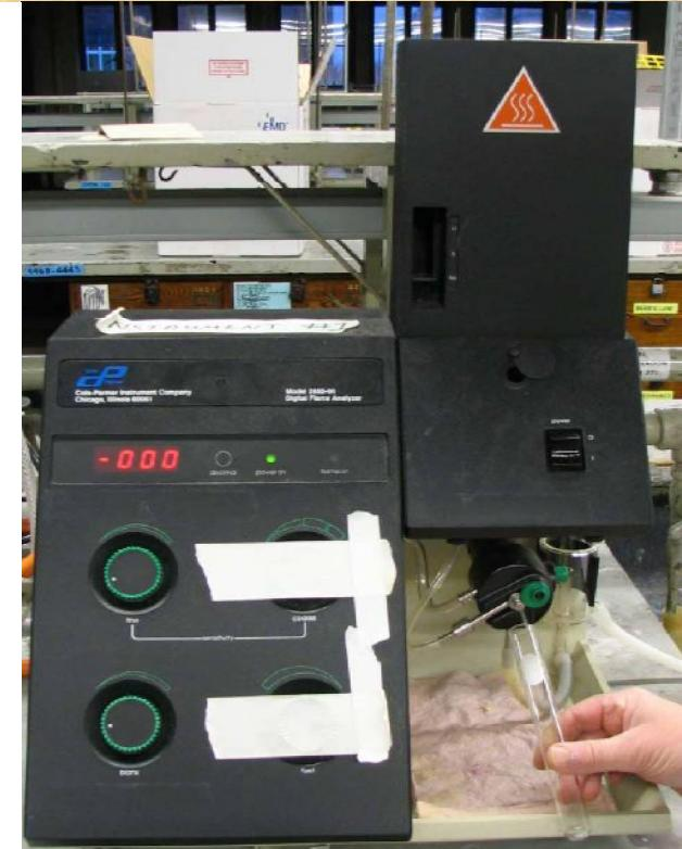
The method is based on the fact that intensity increases linearly with the  $\text{Na}^+$  concentration
